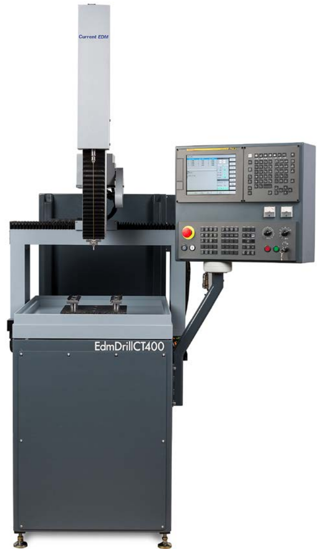
CT400 3 Axis with FANUC 0i-MF Plus CNC Controller
